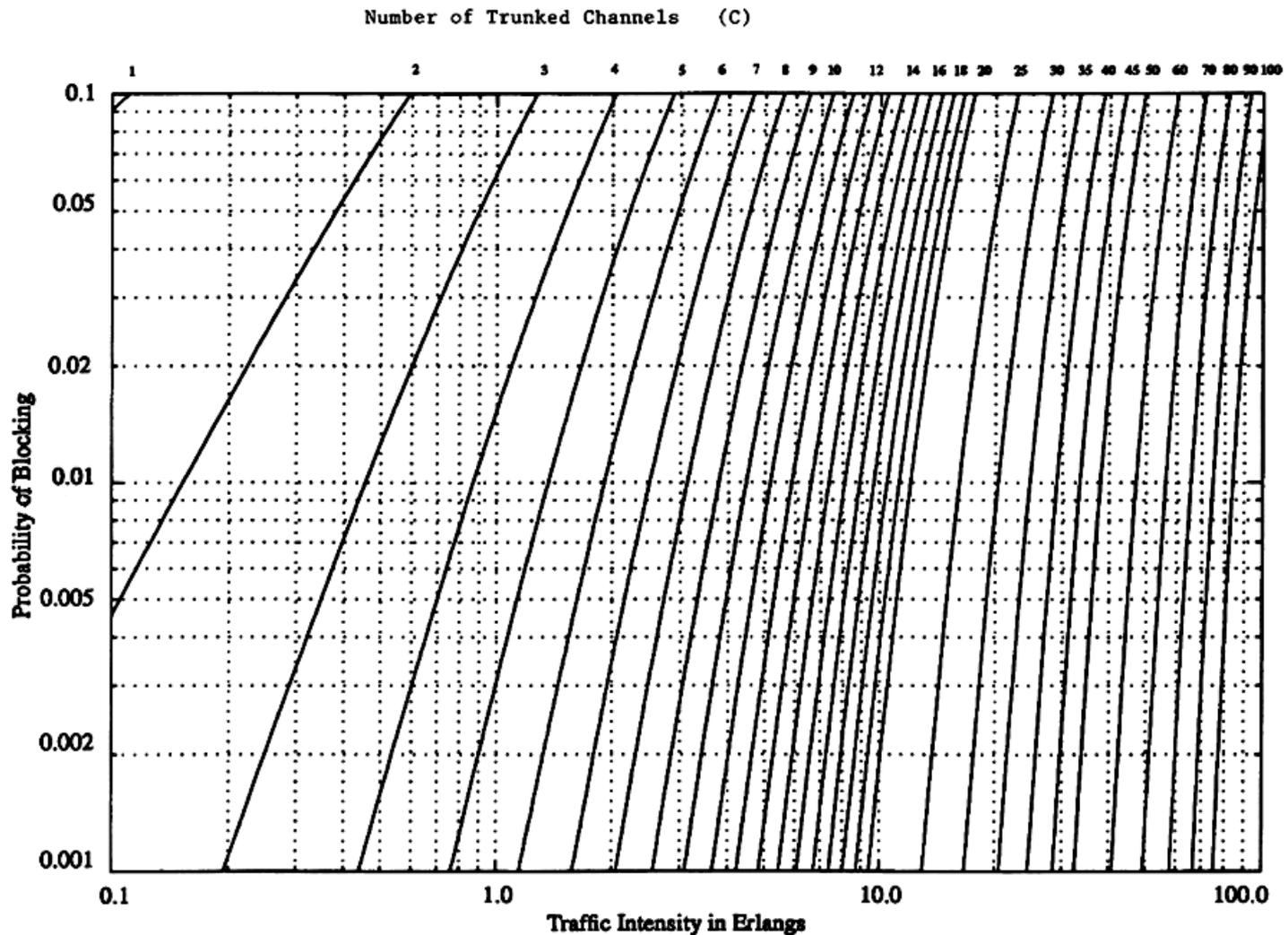
Figure 3.6 The Erlang B chart showing the probability of blocking as functions of the number of channels and traffic intensity in Erlangs. 0
